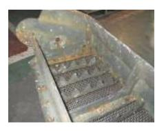
Biofoul four years earlier, was found to be growth free except on uncoated areas such as around fixing nuts and bolts. Just these areas were therefore coated in Biofoul at the time.
