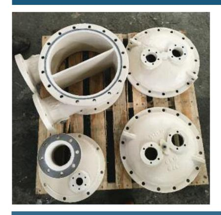
Corrocoat USA provides a wide array of corrosion solutions for the Crowley Maritime Corporation. A typical recent project was to corrosion protect three sets of severely corroded condenser heads and water boxes and their associated piping.
