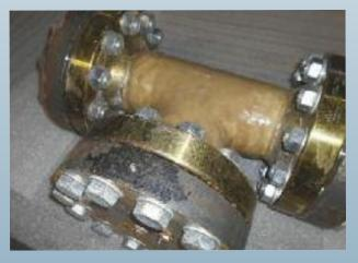
Materials Research Laboratory. The CSR system uses a combination of Corrocoat specialist coatings interlayered with GRP composite laminates to repair, corrosion protect and give structural strength to pipework and other equipment, at a fraction of the cost and inconvenience of replacement. It is an ideal solution for capital process equipment where corrosion has reduced the wall thickness to below an acceptable minimum or where damage has occurred.
