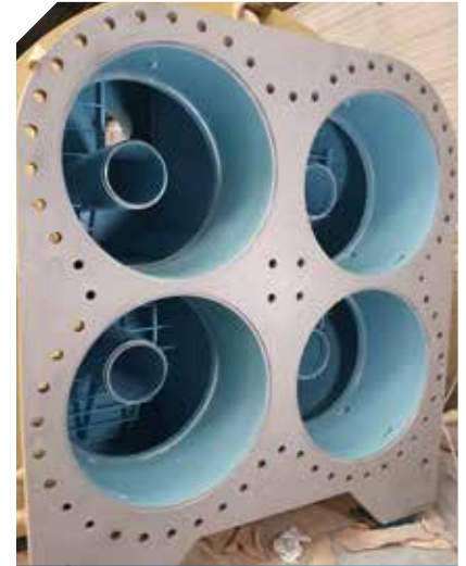
Cooling water area following protective coating
